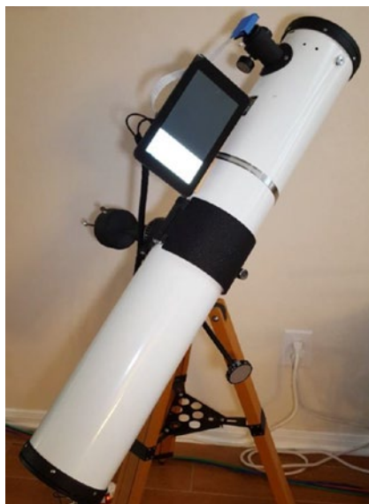
Figure 7-15. 4 1/2-Inch Reflector with Raspberry Pi
