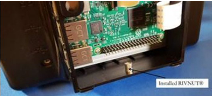
Figure 7-25. RIVNUT Installed in the Case
