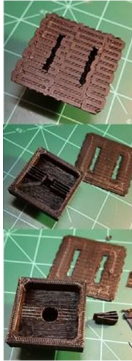
Figure 7-31. Cleaning Up the 3D Printed Camera Case
